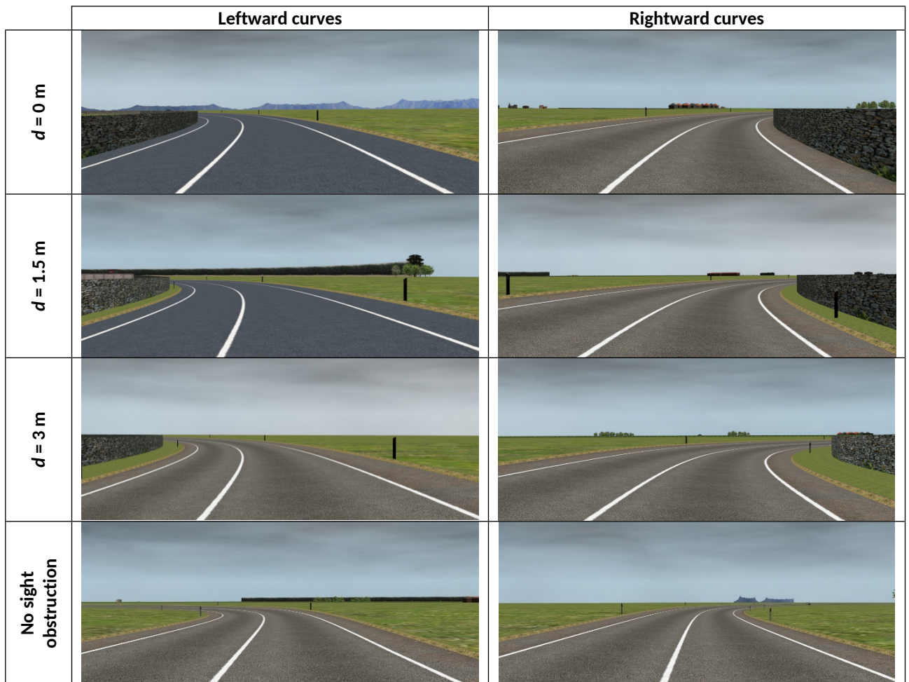
274 Figure 4. Frames of right-hand and left-hand curves with sight obstructions at a distance d equal to 0, 1.5, 3 m, and 275 without the lateral wall. Road delineators were included in accordance with the Italian Highway National Code 276 (MIT, 1992). 277
