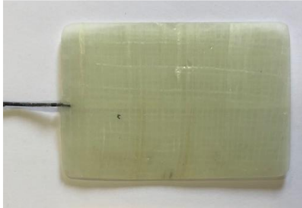
Figure 4. 28. Picture of epoxy sample where two OFSs are embedded. b) Picture of GFRP sample with one embedded OFS.
