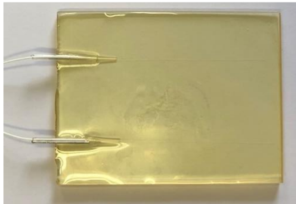
Figure 4. 19. a) Picture of epoxy sample where two OFSs are embedded.
