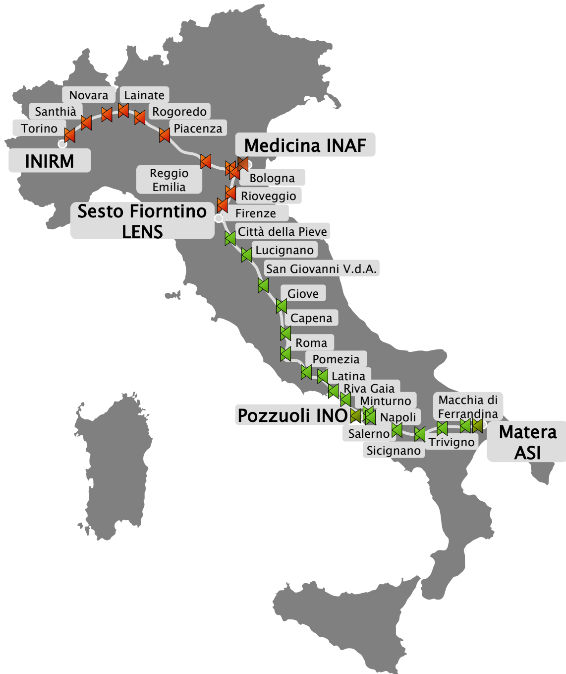
Figure 2.4: The map shows the position of the EDFAs installed along the link backbone. The orange EDFAs were installed back in 2014, while the green EDFAs have been installed last year for the link extension. All the amplifiers are housed in telecom shelters except for the dark-orange and dark-green EDFAs which are placed in the laboratories at the span terminals.
