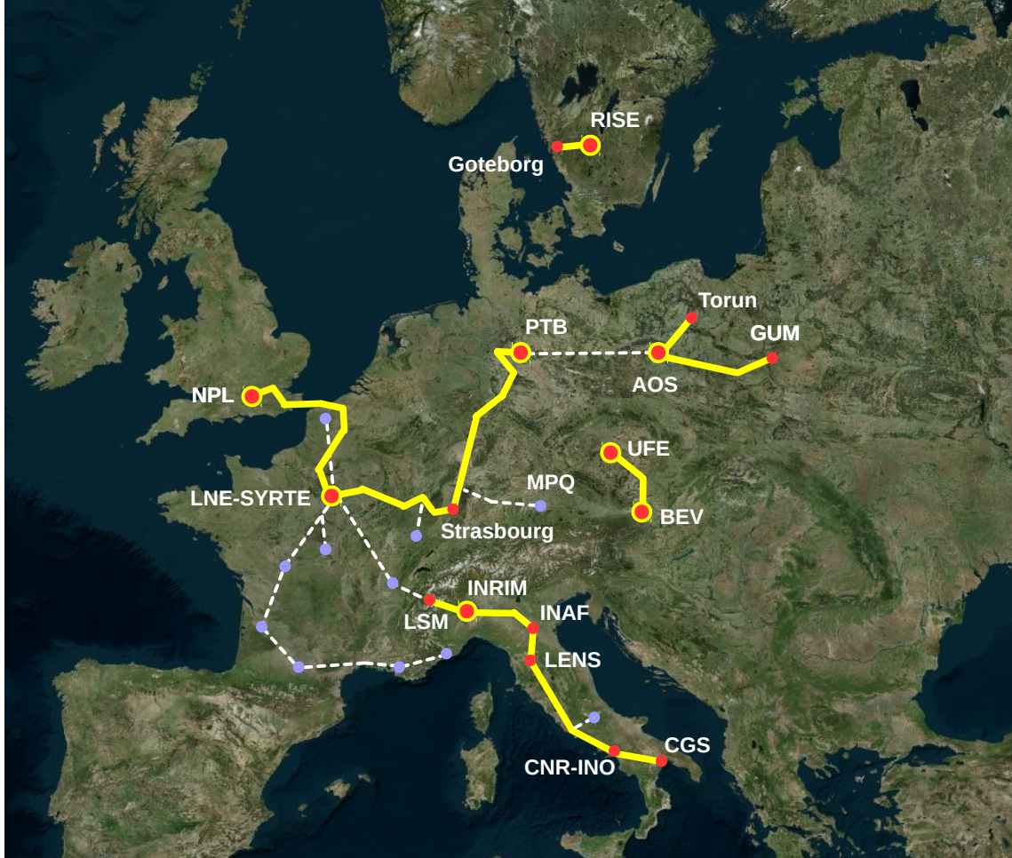
Figure 1: Yellow line: operating links. INRIM-INAF-LENS [30, 31], INRIM-LSM [32], LNE-SYRTE-PTB [33], LNE-SYRTE-NPL [34], Torun-AOS-GUM [35], SP-Goteborg [36], UFE-BEV [37]. White dashed lines: links under development within the OFTEN project.
