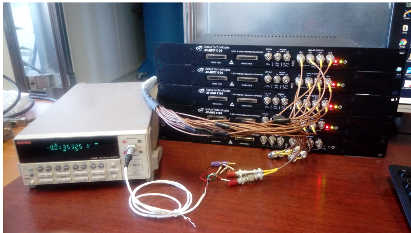
Figure 5.9: Photograph of the instrumentation controlled by the software: on the right, five AT-AWG 1104 (four are used to drive a 13-bit PJVS), on the left, the Keithley 2182A nanovoltmeter for measuring the PJVS output voltage.
