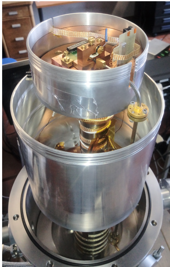
Figure 5.15: PJVS cryopackage installed on the PT cryocooler coldplate. The Si diode temperature sensor and the WR-12 waveguide for the rf transmission are shown as well.
