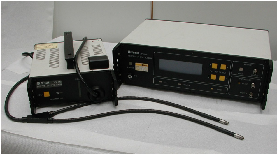
Fig. A.16 Differential laser polytec sensor head with vibrometer controller
