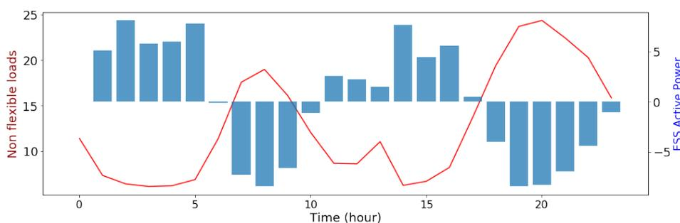
Figure 8: Storage system schedule vs. downstream loads.
