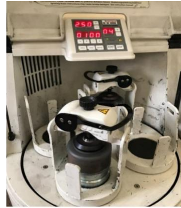
Fig. 1: SWC Biochar - Grinding operation with planetary multi-station mill
