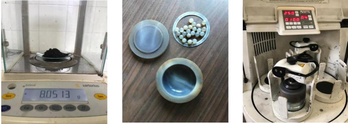
Fig. 1: SWC Biochar - Grinding operation with planetary multi-station mill
