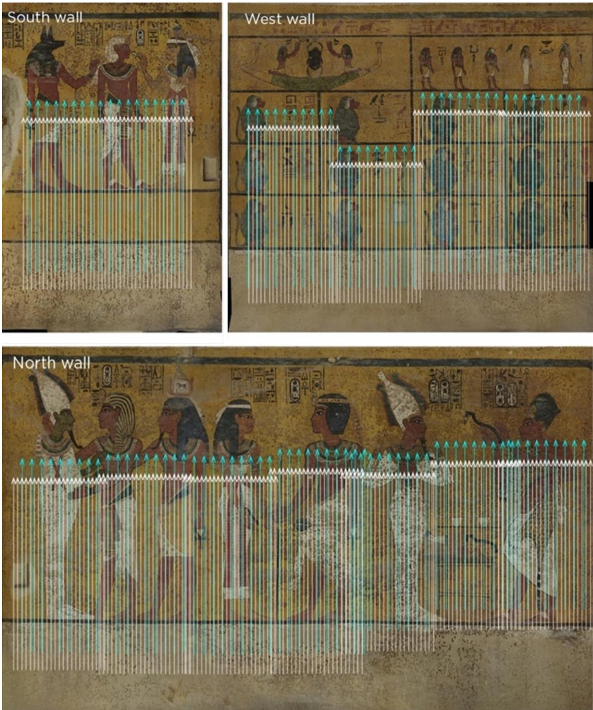
Figure 3S: IF radar profiles acquired with the multi-channel IDS Stream-C system along the KV62 walls, white arrows represent the position of the radargrams acquired in TM-mode, at fixed spacing of 0.0435 m; cyan arrows represent radargrams acquired in TE-mode at fixed spacing of 0.099 m.
