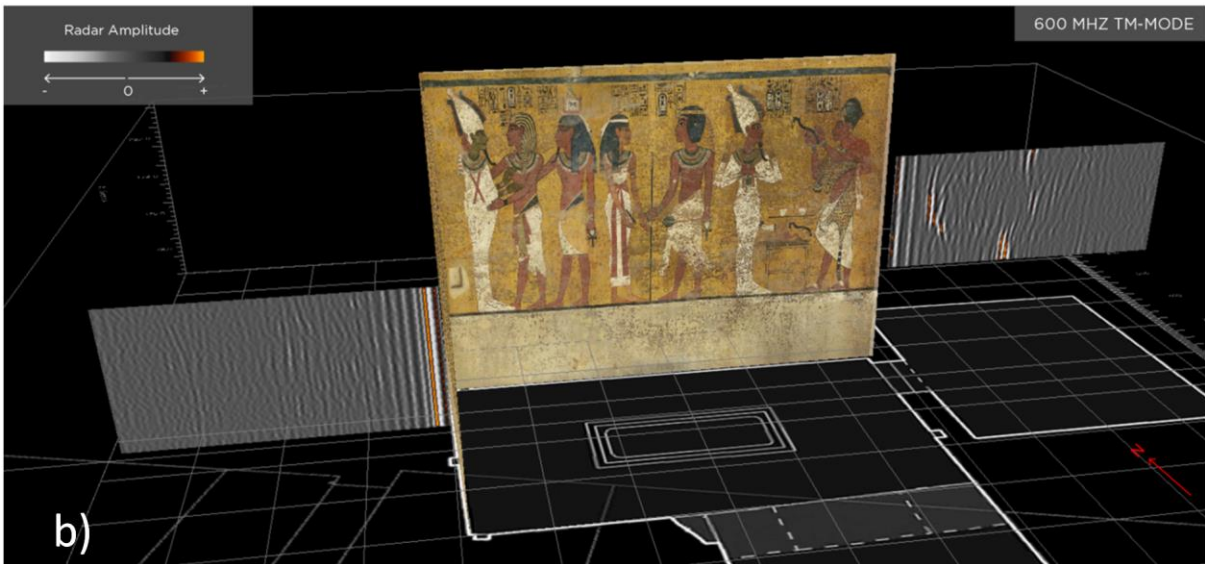
Figure 6: IF processed data: perspective view of IF scans showing the response recorded from: a) the North, East and South walls and b) from the East and West walls.
