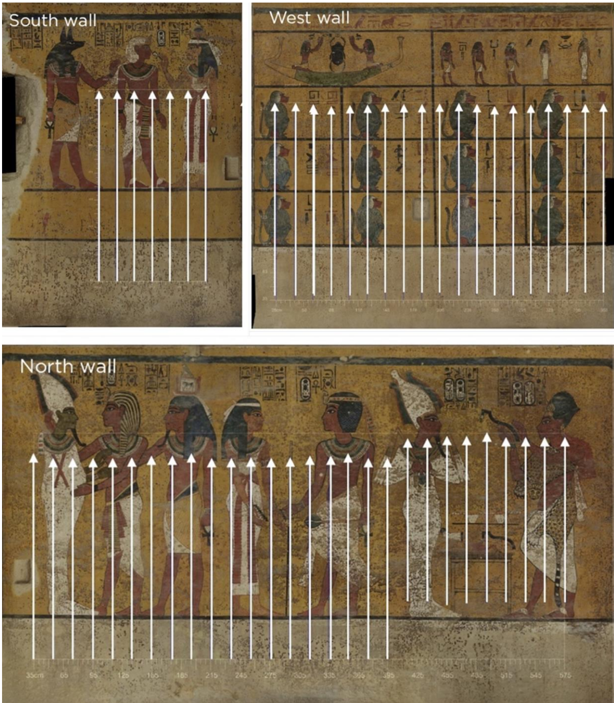
Figure 2S: LF radar profiles acquired with the IDS TR200 GPR unit along the KV62 walls, the spacing among the lines is of 0.2 m.
