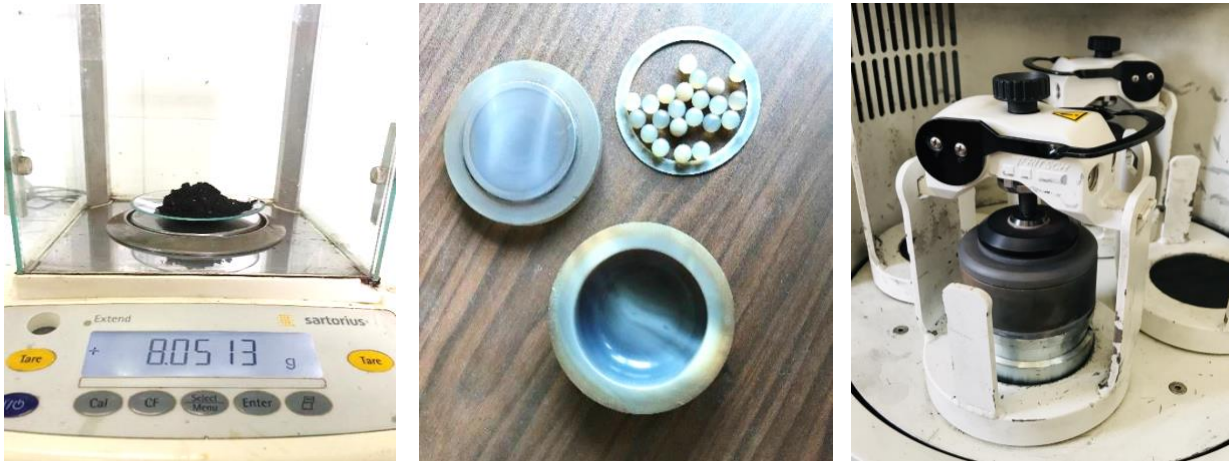
172 Fig. 1: SWC Biochar - Grinding operation with planetary multi-station mill
