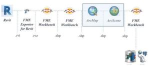
Figure 8. FME Workspaces: from IFC to shapefile.
