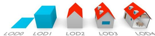
Figure 1. Level of Detail for CityGML standard.
