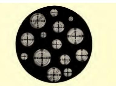
FIG. 121.—Doubly Refracting Liquid Crystals of Cholesteryl Acctate, projected on the Screen in the Act of Growth (see p. 281).
