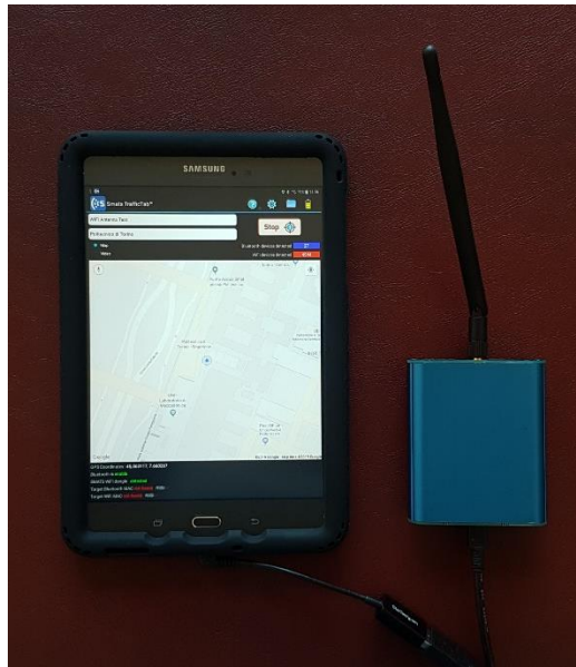
Fig. 70 Tablet TrafficTab SMATS with Wi-Fi antenna
