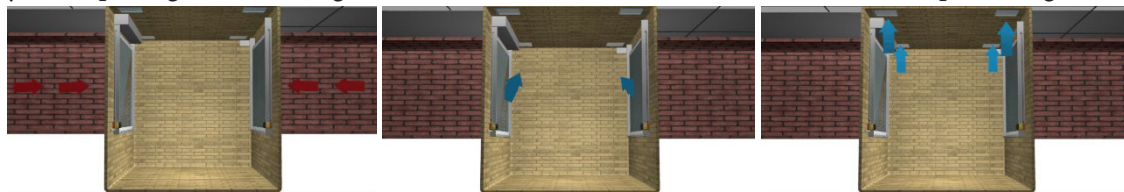
[Figure 2] Air flow through the windows composed by three cellulose pads in the technical room placed at the basement of the building.
