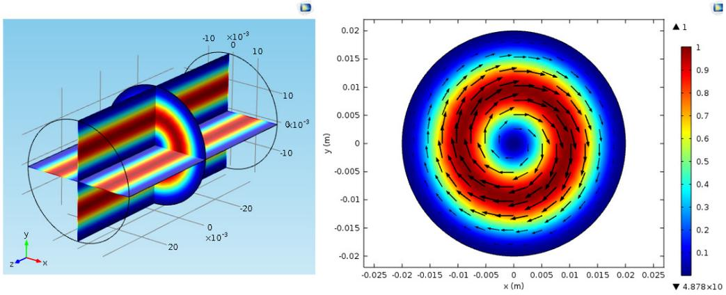
**Figure 2.** Normalized electric field intensity for the superposition  $TE_{c01} - iTE_{s01}$  evaluated with the software COMSOL Multiphysics in a circular waveguide of radius  $a = 0.02$  m. The real part of the vector field over the middle transverse cross section is also reported.
