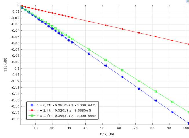
**Figure 7.**  $S_{21}$  parameter as a function of the guide length  $z$  for a circular waveguide with copper walls and radius  $a = 0.02$  m. In the legend the results of the corresponding linear fit:  $S_{21} = -2\beta_{nj} + c$ , with  $c \approx 0$ , are also reported.
