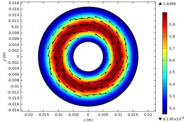
**Figure 5.** Normalized electric field intensity for the  $n = 0$  TE superposition evaluated with the software COMSOL Multiphysics in a coaxial cable filled with Teflon. The real part of the vector field over the middle transverse cross section is also reported.
