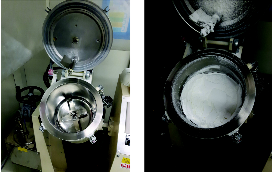
Figure 9.1: Photos of the turbo mixer and of the obtained PVC-P blend
