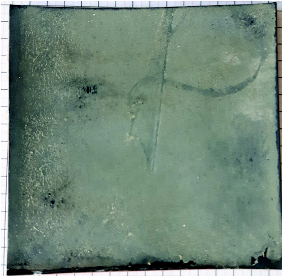
Figure 8.5: Photo of one of the specimens aged for 90 days at 45°C where fungi appeared
