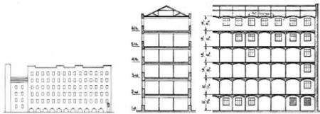
Figure 2.1. Silk mill in Derby (1718). Figures extracted from: Ackermann, *Building for Industry*, 17.
