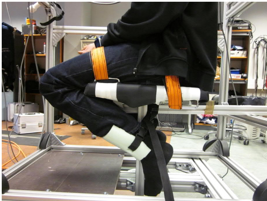
FIGURE 13 The three eyelets in front were used to fixed athletes' thighs, whereas the two in the back were used to tighten athletes' pelvis by means of two belts
