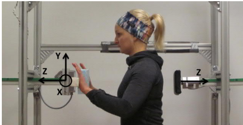
FIGURE 19 First maximal voluntary force tests: simulated bench press without back support
