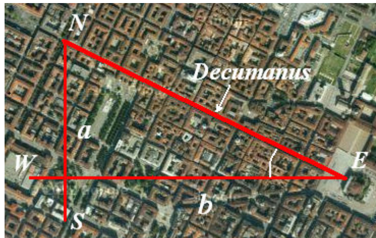
Fig.2 The decumanus is the hypotenuse of the triangle. Measuring a and b we find the angle. From the figure we have an angle of 25.8 degrees.
