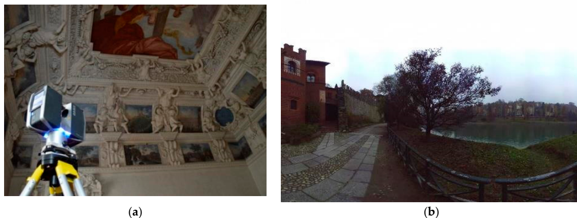
Figure 3. Terrestrial Laser Scanner (TLS) by FARO®: (a) The FARO® Focus 120 during the acquisition and (b) planimetric view of an outdoor coverage range of an X330 scanner.
