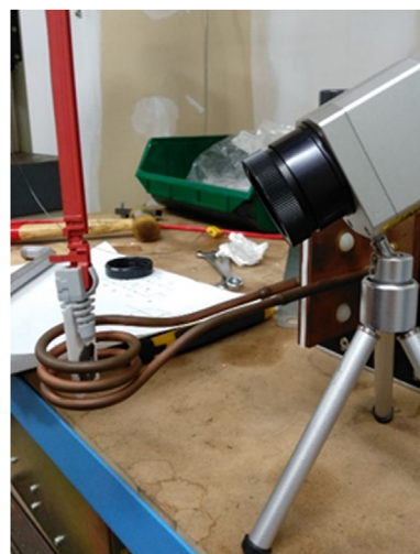
Fig. 17. Experimental set-up of the temperature measurement.
