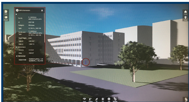
Fig. 6. Alphanumeric properties visualization of the BIM model through Virtual Reality (graphic elaboration by the authors).
