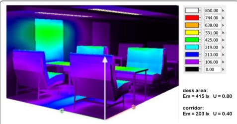
**Fig. 9** Results of lighting simulations for a sample train coach. Average illuminance ( $E_m$ ) and uniformity (U) over the table and over the corridor (luminous efficacy:  $\eta = 39.9 \text{ Im/W}$ )
