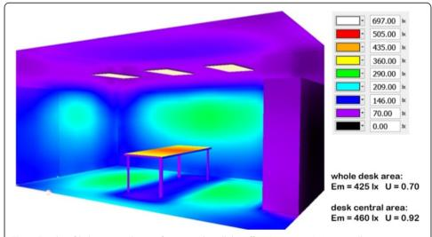
**Fig. 7** Results of lighting simulations for a sample cellular office (5 m \* 3 m). Average illuminance over the desk ( $E_m$ ) and uniformity (U) using the luminous efficacy value measured in laboratory for the prototype ( $\eta = 39.9 \text{ lm/W}$ )
