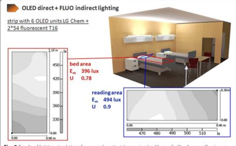
**Fig. 8** Results of lighting simulations for a sample patients' room in a health care facility. Average illuminance  $(E_m)$  and uniformity (U) over the bed and over a reading area (luminous efficacy:  $\eta = 39.9$  lm/W)
