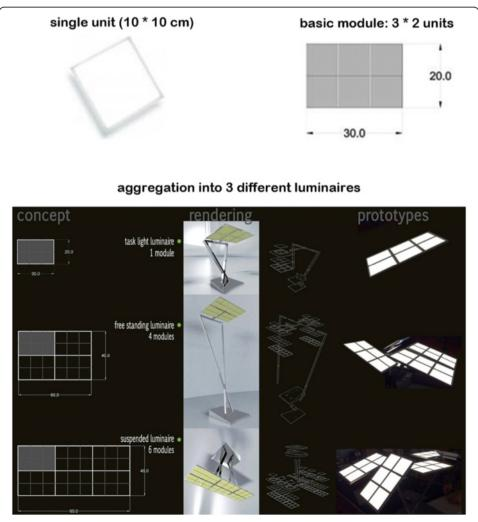
**Fig. 3** Different aggregation of the OLED module to create 3 different luminaires. A ceiling-suspended, a free-standing and a task lighting were created
