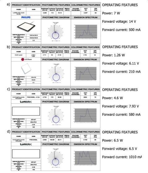
**Fig. 1** Performances measured for some of the OLED units which were tested: **a** Philips Lumiblade GL350; **b** LGChem LG6S1; **c** Lumiotec P05 Series; **d** Lumiotec P06 Series
