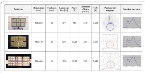
**Fig. 6** Summary of performances measured in laboratory on the luminaire prototypes. Note: measurements were taken in the absence of the secondary optics which was studied in the project
