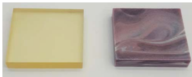
Fig. 2. Fresnoite glass (left) and glass-ceramic (right)
