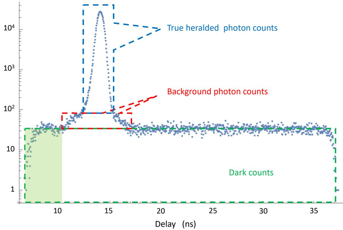
**Figure 2.** Histogram of the detections acquired in one run by one of the INRiM HBT gated SPADs, with a 30 ns detection window. The true heralded photons (Her), background photons (Bkg) and dark count (Dark) contributions can be clearly seen. The green shaded area indicates the dark counts forbidding the SPAD to detect a photon from the HSPTS.
