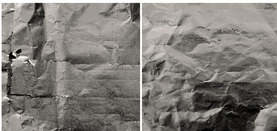
Figure 4. 2: Backside of HCl doped PANi@C/S composite coated Aluminum foils a) 3 times DI water and 3 times alcohol washed b) extensively washed with the bulk of DI water
