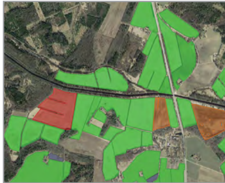
Mowing detection results are presented on a public web map of Lääne-Viru County. Green represents mowed area, red not mowed area and orange late mowed area.
