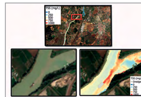
Sentinel-2 image showing the turbidity plume generated during the dredging operations in the Guadalquivir estuary and Port of Seville and map of Suspended Solids in November 2016.
