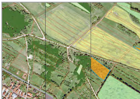
Monitoring of afforestation for a test site in the forest district Hainich-Werratal (from the left to the right): forest mask in green, areas already recognised as forest in light green, new forest areas in orange, orthophotos in the background.
