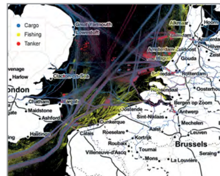
Distribution of AIS messages which are used to teach the system how to automatically recognize different ship types.
