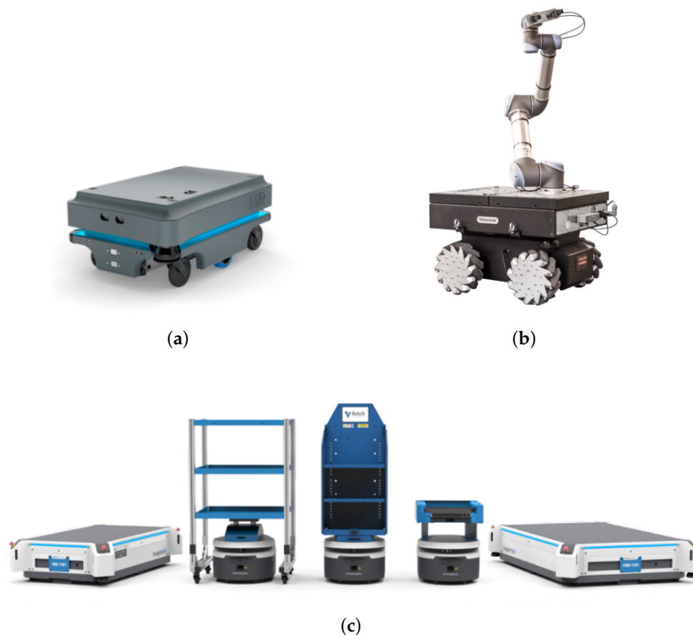
Figure 18. Examples of AMRs. (a) The MiR200 is a safe, cost-effective mobile robot. It can be equipped with customized top modules, including lifts, bins, and cobots [45]. (b) The RB-KAIROS is a completely integrated Collaborative Mobile Manipulator (CMM), designed for the development of industrial tasks [46]. (c) Fetch robot AMRs’ collection [47].
