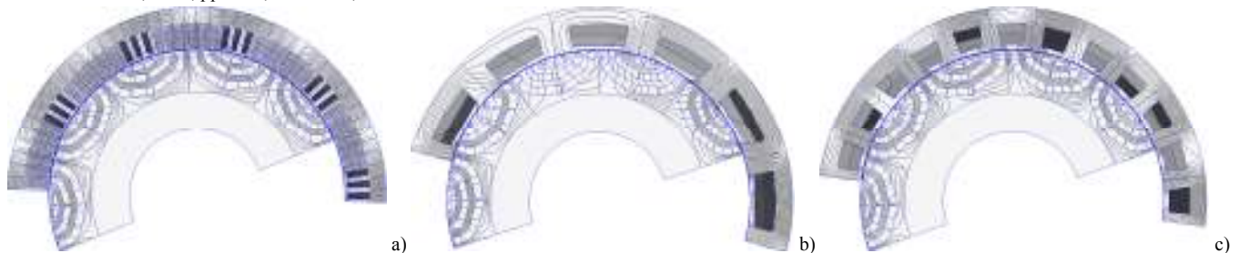
Fig 22. Flux density contours for the three PM-SyR machines supplied with d -axis current only. a) q = 3 ; b) q = 2/5 ; c) proposed q = 4/5 solution.
