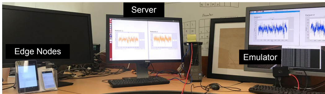
Fig. 2.12 The implemented system for EEG telemonitoring.
