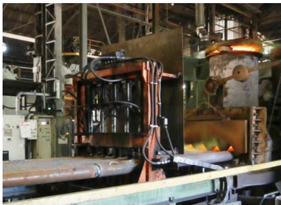
Figure 1. Special pneumatic track system used to move the steel bars.
