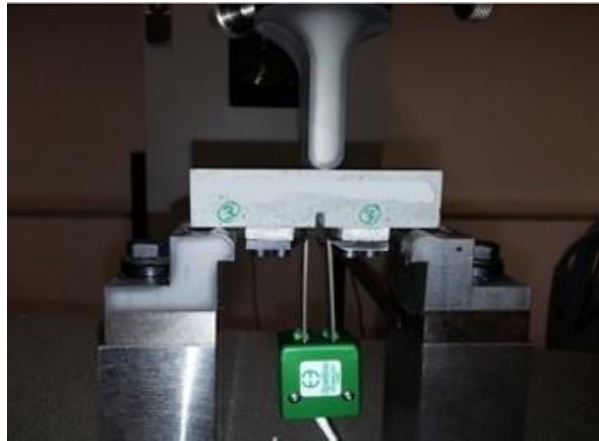
Figure 28: Prismatic sample of cement composite tested with the single-column ZwickLine z050 flexural testing machine having maximum load capacity of 1 kN. The CMOD (Crack Mouth Opening Displacement) control mode was selected and the displacement rate was fixed as 0.003 mm/min for all the specimens
