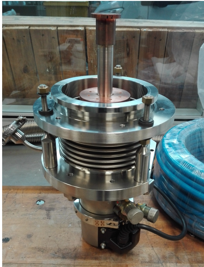
Figure 41: A Leybold 5/100 cryocooler joined with a bellows flange.
