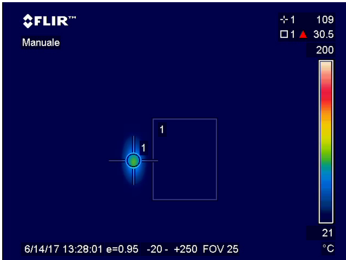
Figure 100: Frame of a video of the heating test performed with an output power of 12 W. The frame is taken after 1 second of irradiation.
