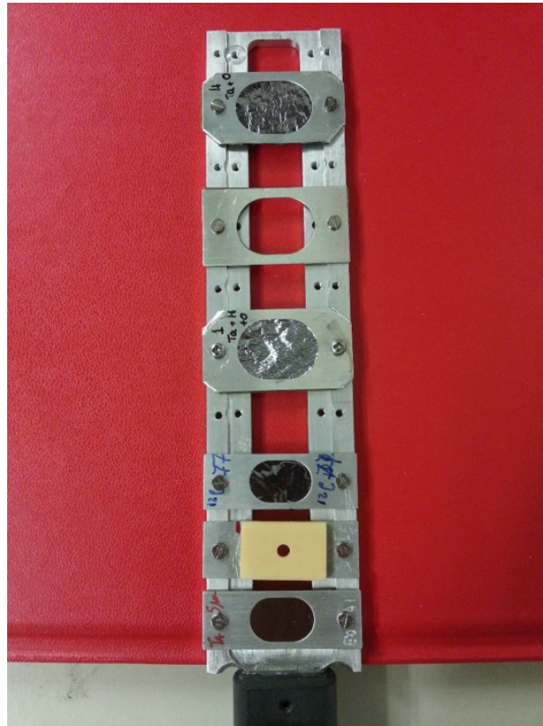
Figure 9: Target used in phases one and two. Materials are deposited on a thin carbon film and held in position by a metal frame. The bottom targets are used for calibration purposes.
