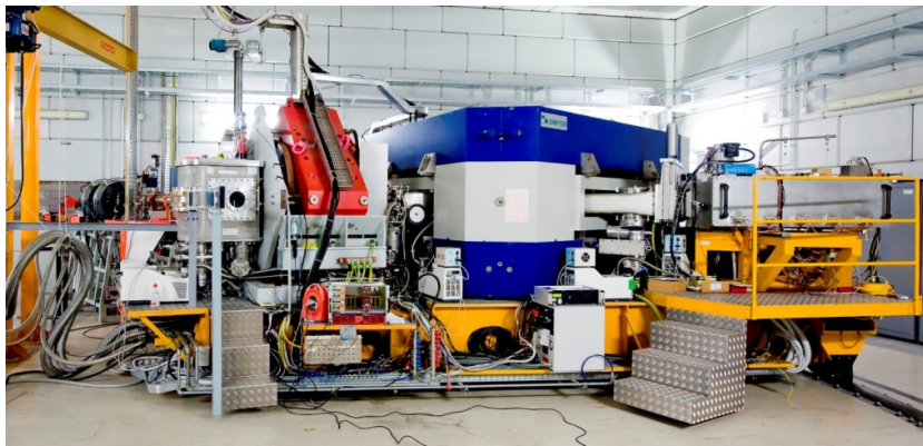
Figure 8: The MAGNEX spectrometer. From the lefthand side, one can see the scattering chamber, the quadrupole (in red) and the dipole (in blue).
