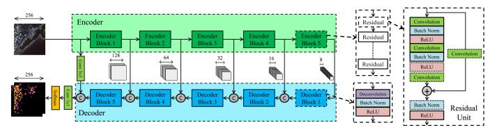
Fig. 1: Proposed encoder-decoder network architecture for satellite image segmentation with exploded residual block and unit diagram and deconvolutional blocks.
