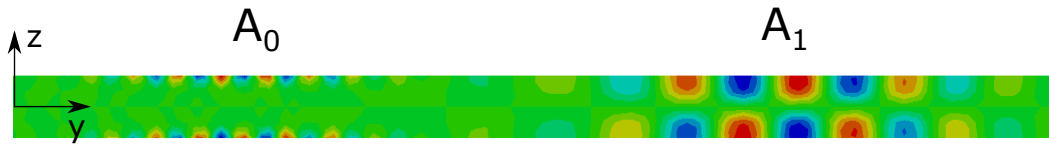
Fig. 10.12 A_0 and A_1 modes at t = 6 \times 10^{-5} for a signal burst of 1.2 MHz.
