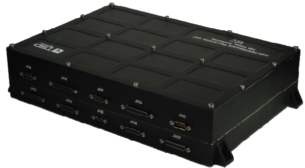
Figure 7: HPHC engineering model assembled in its cabinet
