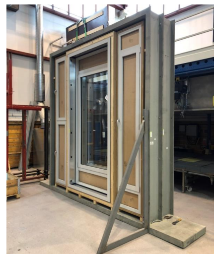
► Fig. 3: View of a sample facade and frame structures for installation in the Climate Simulator
