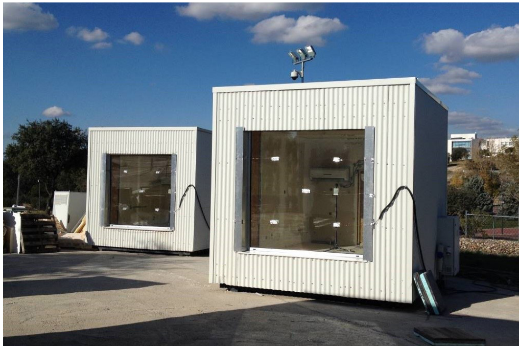
Figure 2 - External cell boxes equipped with radiant glass façade in UPM Campus.
