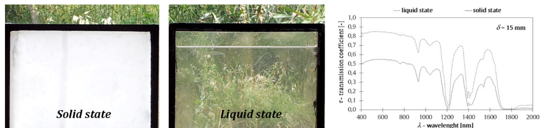
Figure 1 - Appearance of a double glazed unit filled with PCM when in solid state (left) and in liquid state (right), together with the spectral transmittance in the solar range for the two states of aggregation. Source: Goia et al. (2015).
