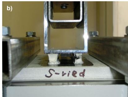
▶ Fig. 2: Experimental test of facade fixing according to ETAG 034 and ETAG 002 performed at Klokner Institute, CTU in Prague
