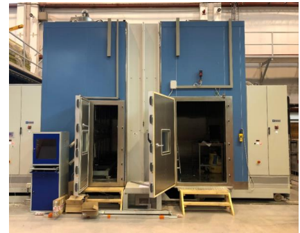
► Fig. 1: External view of the Climate Simulator, with the outdoor cell on the left-hand side and the indoor cell on the right-hand side
