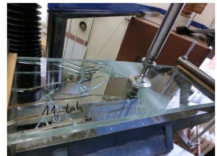
▶ Fig. 3: Non-standard connection tests of the façade glass panel performed at Klokner Institute, CTU in Prague
