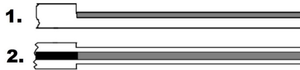
Figure 1. Sample layout: 1. Beam damped one side, 2. Sandwich layout
