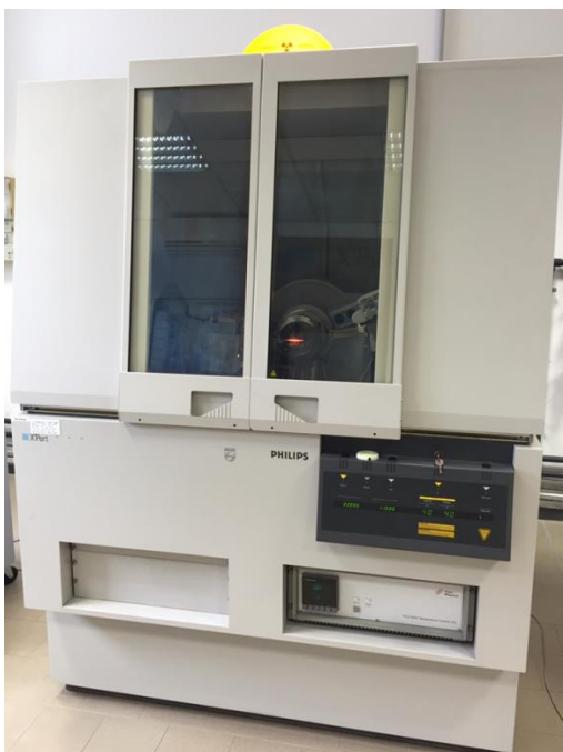
Figure 3.12 XRD analyzer (Philips X'pert) used at Polytechnic University of Turin.
