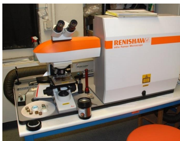
Figure 3.14 Renishaw inVia Reflex micro-Raman spectrophotometer at Polytechnic University of Turin.
