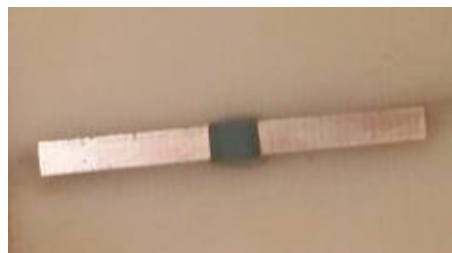
FIGURE 1: Examples of carbon film obtained using screen printing technique.
