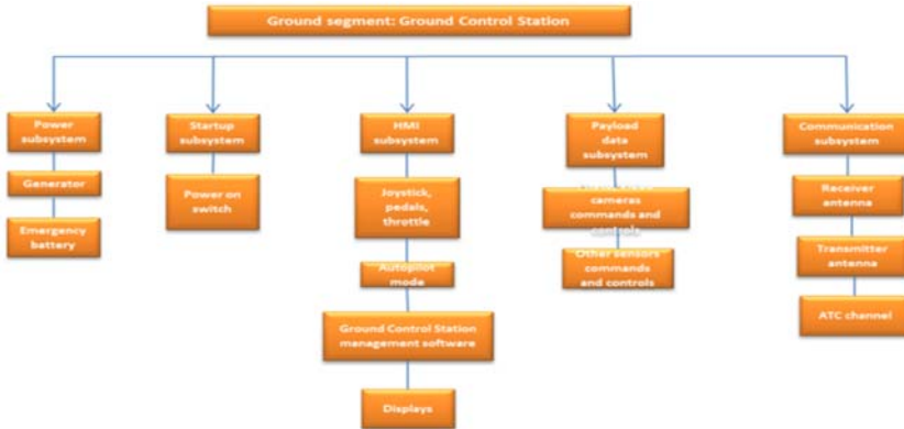
Fig. 3. RPAS model, ground segment.
