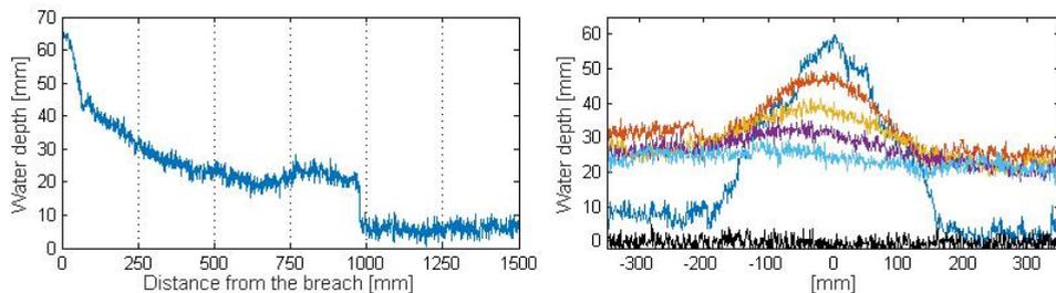
**Figure 4:** On the left: water depth along the breach axis at time 1 s after the opening (Configuration A). On the right: water depth along sections parallel to the gate, starting from the upper line, respectively 1, 10, 20, 30, 50 and 150 cm downstream the breach at time 1 s after the opening (Configuration A)
