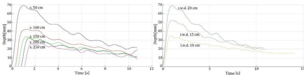
**Figure 5:** On the left: configuration B with initial water depth at breach 20 cm. Mean value of the water depth in squared clusters of edge 10 pixel set respectively at 50, 100, 150, 200, 250 cm downstream of the breach. A low-pass filter is applied. On the right: comparison between the 3 "configuration B" realisations of the mean value of the water depth in a squared cluster of edge 10 pixel set 50 cm downstream of the breach. A low-pass filter is applied.
