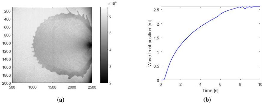
**Figure 3:** On the left side an image acquired by the camera during the experiment (down-stream slope  $0^\circ$ ). On the right: time of arrival of the water front at different section down-stream the plane.
