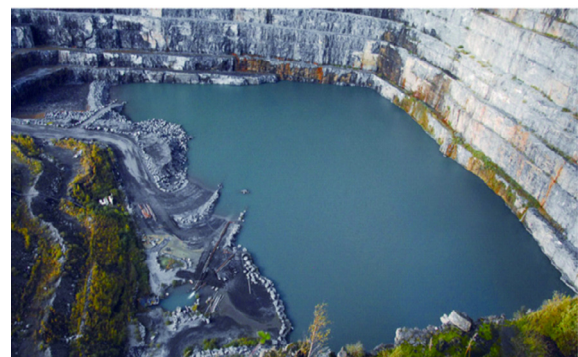
(c) Exhausted quarry pit in which the overburden has to be disposed
