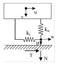
Fig. 1. Node-to-node contact element.
