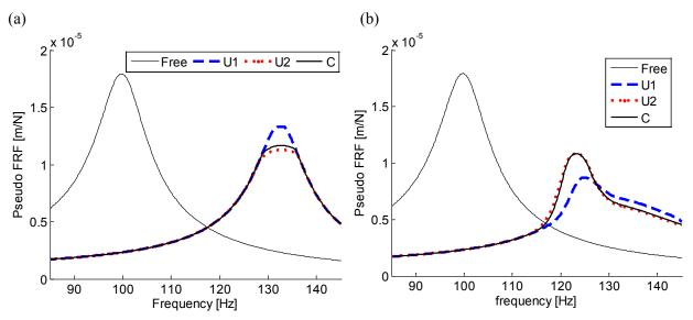
Fig. 11. Pseudo-FRFs comparison for different  $F_{pl}/F_{exc}$  ratios: (a)  $F_{pl}/F_{exc}$ =84, (b)  $F_{pl}/F_{exc}$ =30.
