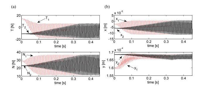
Fig. 13. Transient response for different initial conditions (U1, dotted curves and U2, solid curves) and common steady state response of the system after the application of a harmonic excitation force: (a) contact forces (steady state:  $T^{(0)}$ = -6 N;  $N^{(0)}$ = 23.9 N), (b) displacements (steady state:  $x^{(0)}$ = -5.4e-5 m;  $y^{(0)}$ = 1.7e-4 m).
