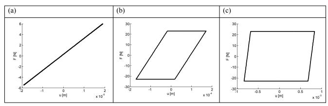
Fig. 6.  $\alpha = 0^{\circ}$ , hysteresis loops for three different resonant responses: (a)  $|F_{exc}|=1$  N; (b)  $|F_{exc}|=24$  N; (c)  $|F_{exc}|=60$  N.
