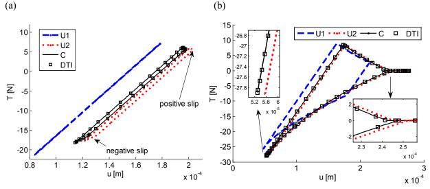
Fig. 12. Hysteresis cycles for the peak frequency U1, U2, C and comparison with DTI: (a)  $F_{pl}/F_{exc}$ =84, (b)  $F_{pl}/F_{exc}$ =30.
