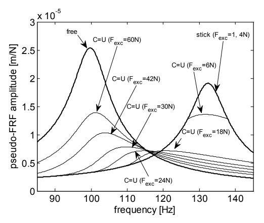
Fig. 5.  $\alpha = 0^{\circ}$ , pseudo-FRFs for different amplitude of  $F_{exc}$ .
