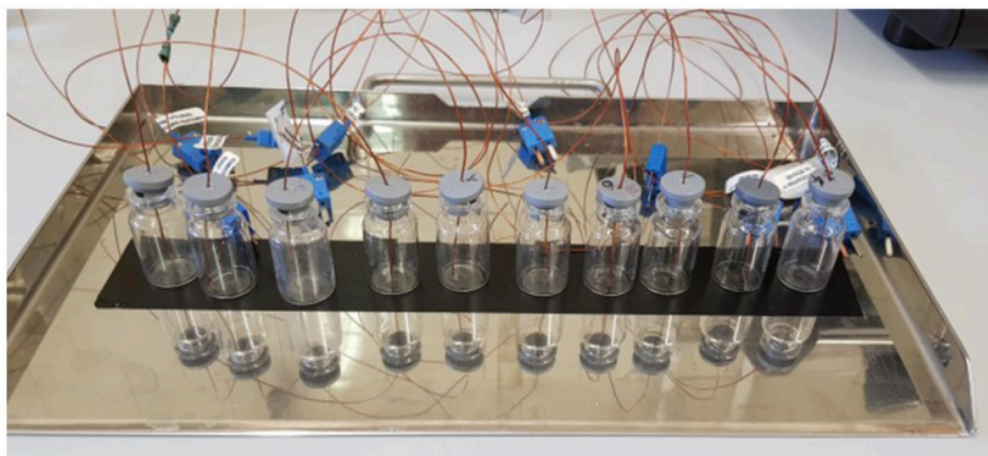
FIGURE 2 | The experimental setup used for testing the thermocouple insertion procedure; here a realization with 10R vials (24 mm diameter) is shown.
