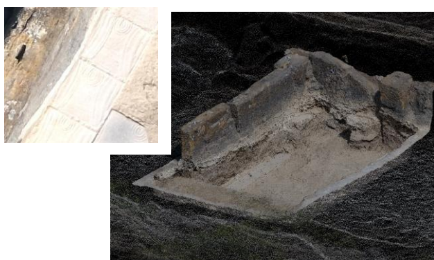
Figure 10. (left) The terracotta paving decorated slabs (from 4 mm resolution orthoimage) (right) A 3D view of the multiscale integrated DSM.
