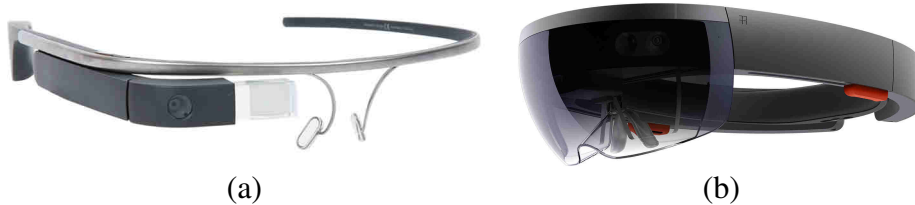
Figure 2.3 AR devices: Google Glass® (a) (credit: Google®) and Microsoft HoloLens® (b) (credit: Microsoft®)
