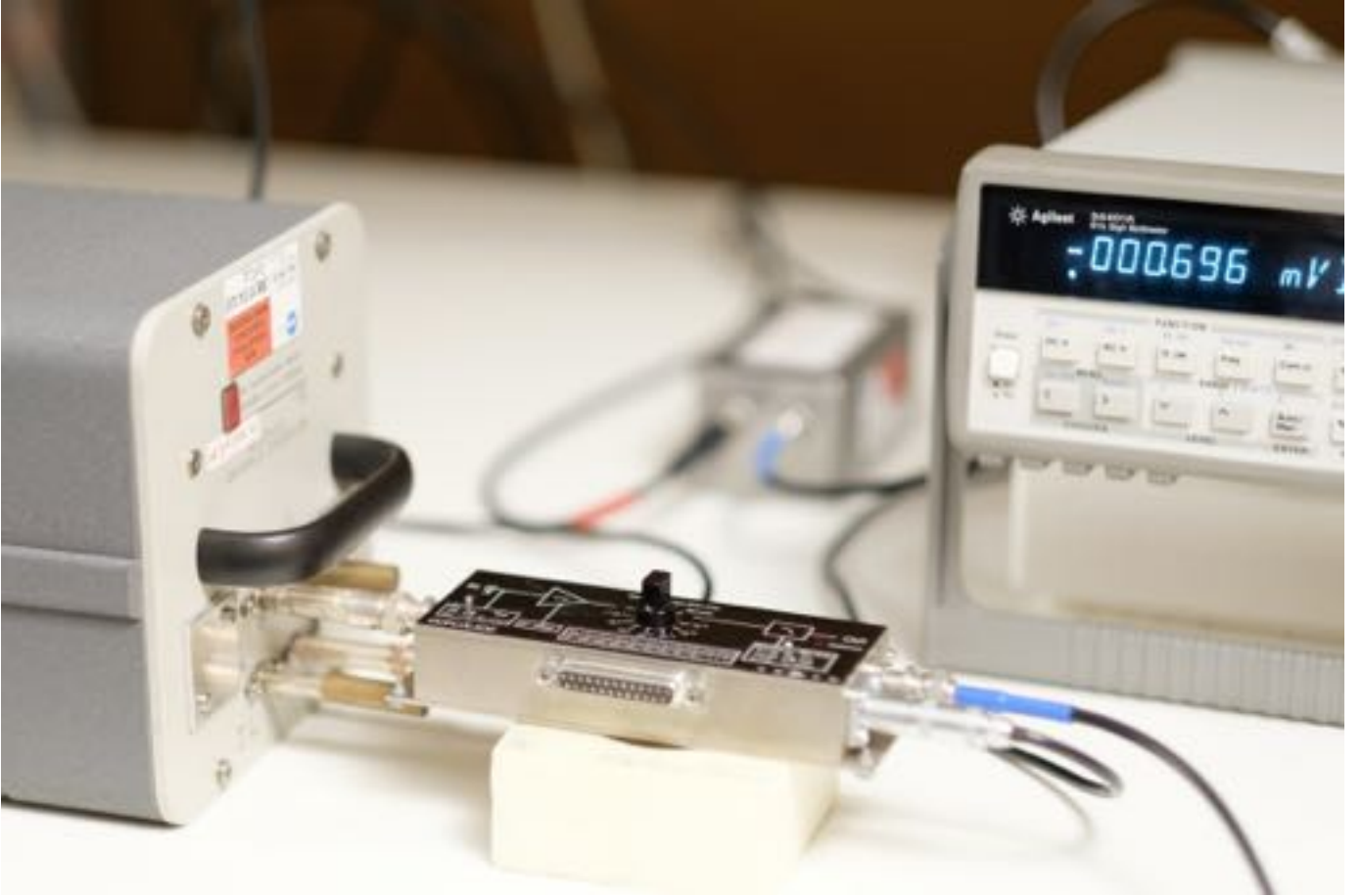
Fig. 4. Detail of setup, showing the direct connection (no cable) of the injection capacitor C (on the left) to the transresistance amplifier A (center of the picture) to minimize currents related to the dielectric absorption in the connection insulators.
