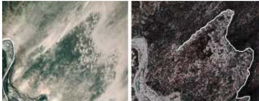
Figure 1 – On the left the dune field in the Google Earth images of 2007. On the right, the same image after processing with the edge detection of GIMP. The front is marked with a white line.
