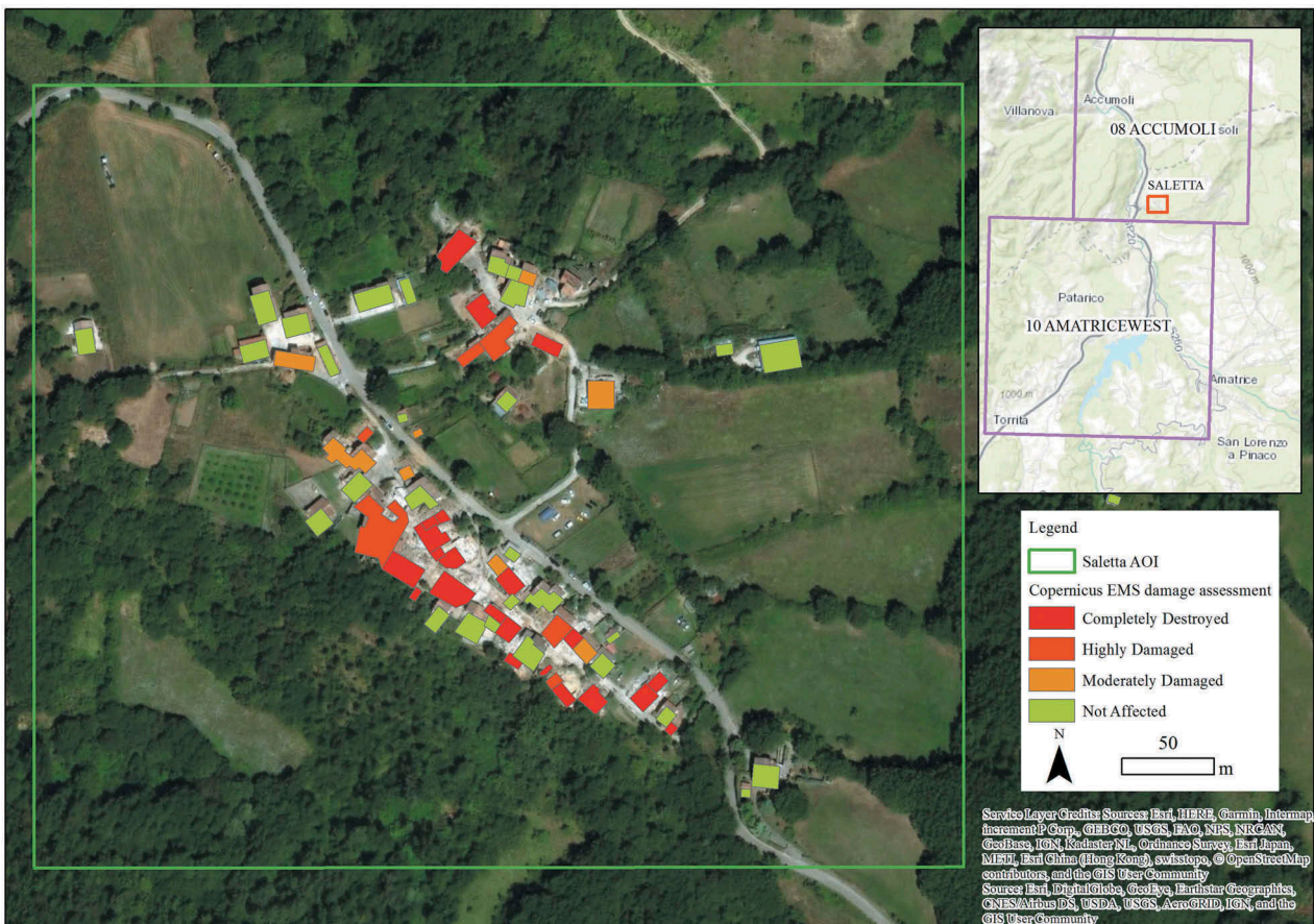
Figure 4. The building footprints over Saletta extracted from [EMSR177] Accumoli: Grading Map, Monitoring 1.
