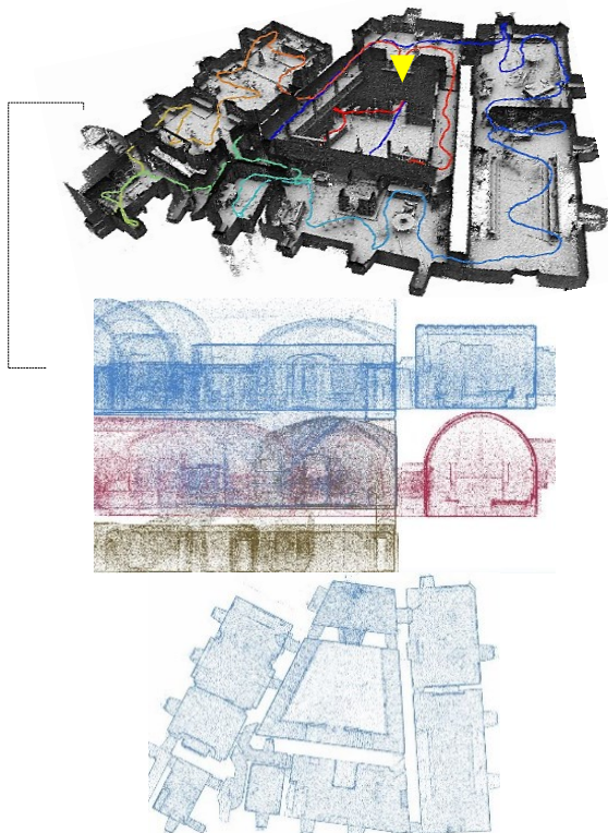
Figure 11. The side-view of the ZEB mapping along the three floors of the Rocca apartments (centre), and planar (down) and 3D view of the first floor (top), and its time-marked trajectory. Starting point at yellow arrow.
