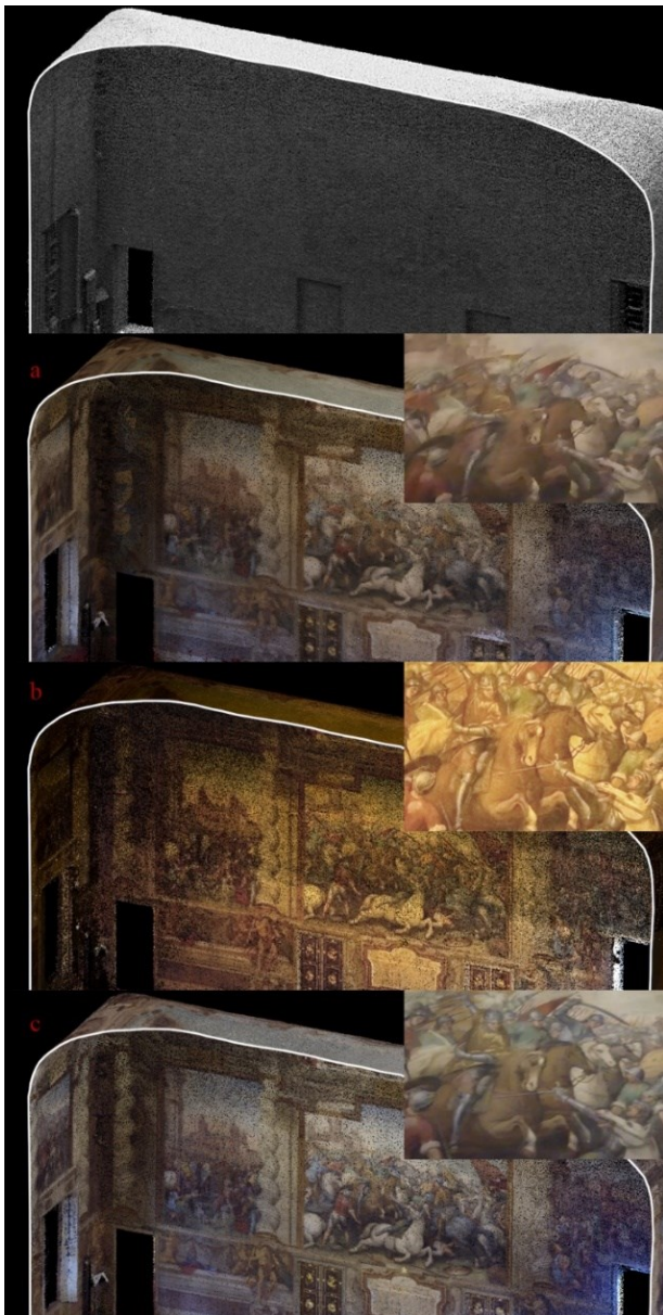
Figure 13. ZEB Point clouds with associated radiometric values: top , ZEB point cloud in shaded view. Photogrammetric point clouds: a , ZEBcam; b , Sony ILCE; c , steadicamera. For each point cloud model, a zoomed view of the image used in the photogrammetric process.
